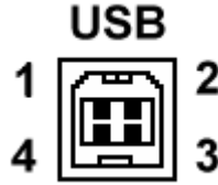
Figure 3-13: USB Connector pin orientation.
